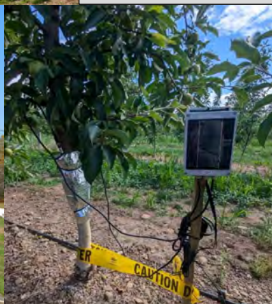
Micro-Irrigation Sensors in an orchard to indicate when irrigation is needed.
