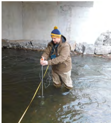
NCSWCD staff measuring velocities (left), filtering water samples (middle), and surveying a cross section (right) of a stream.
