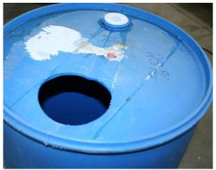
4. Cut a 6 inch diameter hole on top off to the side. Position the hole so the gutter can be placed over it.
